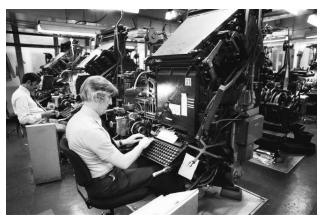
reporters' stories line by line into rectangular pieces of molten metal piecing together entire lines, stacked together to form columns to form pages.
